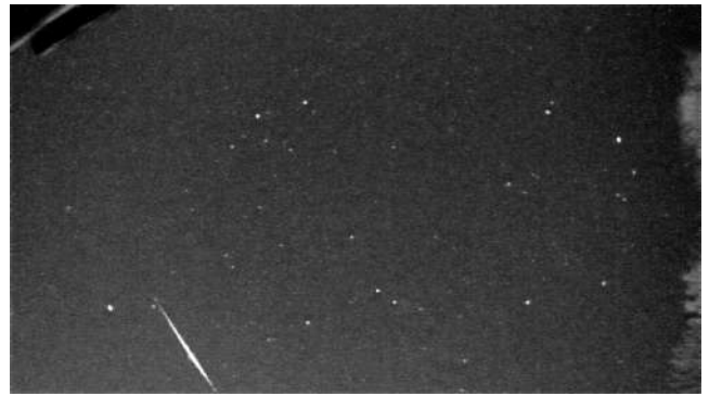
Figure 6 – A meteor captured with the IMX225 CMOS camera. Visible constellations are Gemini (centre) and Auriga (right). The image is a 10.24 s maxpixel obtained using the Four-frame temporal pixel compression method.
